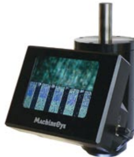
A video image shows a machinist's ruler with 1/2 millimeter rulings. Source: MachineEye
