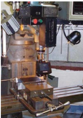
The MachineEye is mounted on a vertical milling machine. It takes approximately 10 seconds to install the unit. Source: MachineEye
